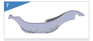
When using this product for the Forticrete Centurion no cut required, for the Redland Fenland and Sandtoft Shire cut leading end on dotted line and for the Marley Anglian cut the solid line.
